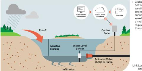
Cloud-based discharge controls rooted in weather forecasting and data from onsite sensors generate saleable credits under a multitude of regulatory markets throughout the country.
